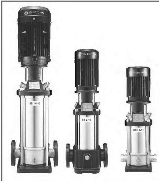
The SB, SBI and SBN pumps are non-self priming vertical multistage pump of in-line design, flange or with Victaulic coupling with equally sized suction and discharge ports. Stage construction with stainless steel impellers, chambers and pressure casing. Pump stub shaft and motor shaft of the IEC-standards motor are directly close coupled. All pumps are equipped with a cartridge type mechanical seal for easy maintenance.
